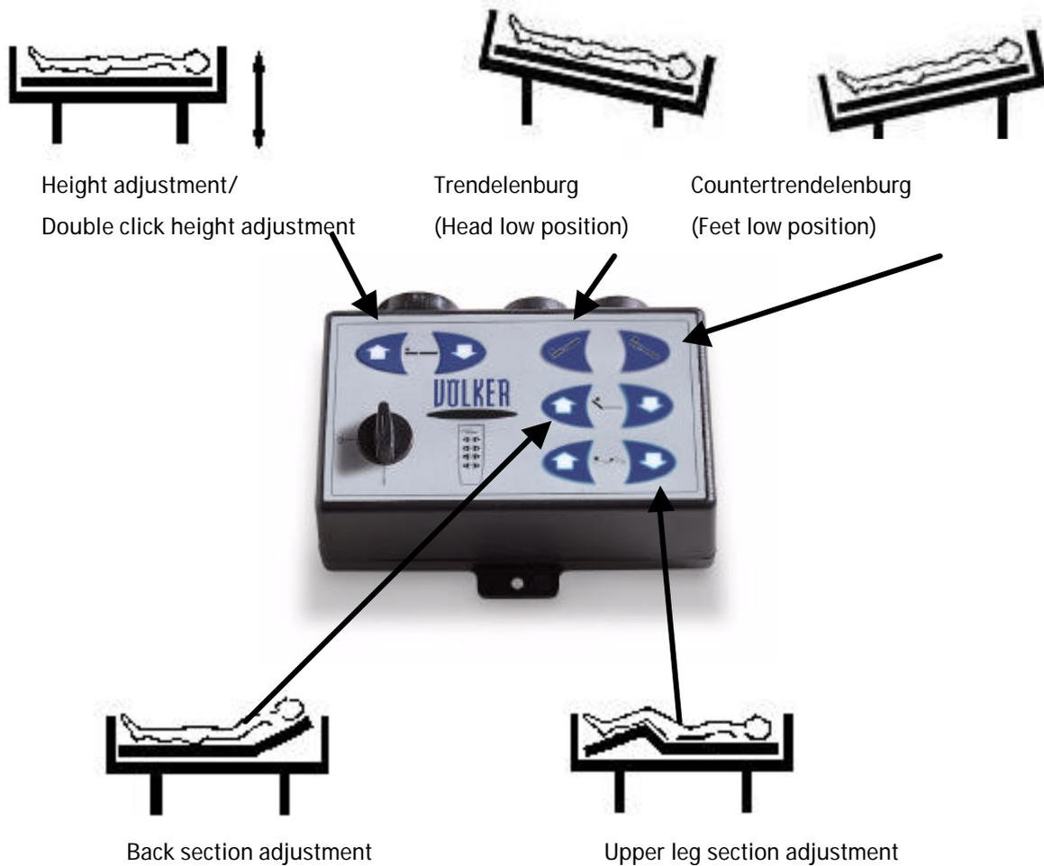
Rotary switch: deactivation of care-receiver's manual control unit and carer's keyboard except Trendelenburg positioning.
