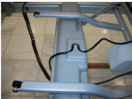
10. Reconnect all plugs to sockets on OKIMAT and replace the socket cap.
