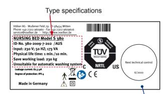
The type label is located on the inside of the head panel.
