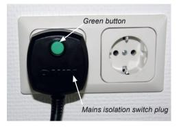
The mains isolation switch ensures that when no electrical function is being actuated, there is no mains voltage to the bed. (Exception: while the battery pack (option) is being charged, there is mains voltage to the bed. This is indicated by a flashing LED on the battery pack).
