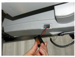
Then pull the contact strip off the battery.
