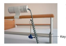
If the nurse keypad is locked, the hand control is also automatically blocked (system lock).
