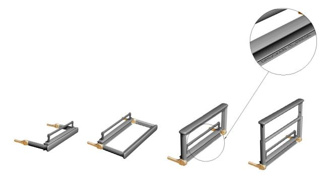
In order to completely fold down an assist rail part, press both buttons on the exterior surface of the frame, right above the cross bar, so that the height-adjustable guard part can be put into its lowest position.
