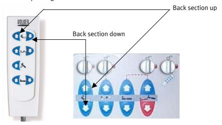
If necessary, unlock the back section using the supervisor control box.
