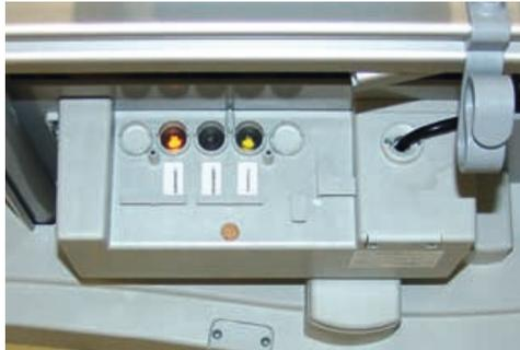
has been connected to the line power, press any button in the hand control in order to make it fully functional again. The battery pack starts a charging cycle when it is connected to the line power after each use, or when the charge has dropped too low.
