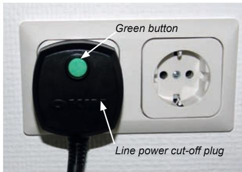
The line power cut-off ensures that there is no line voltage supplied to the bed when no electrical bed function is being operated. (Exception: During charging of the battery, the bed is supplied by line voltage. This is indicated by a flashing LED at the battery pack).
