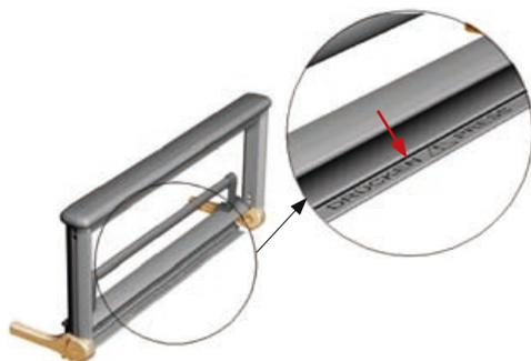
3. Push the side rail in completely under the lying surface.
