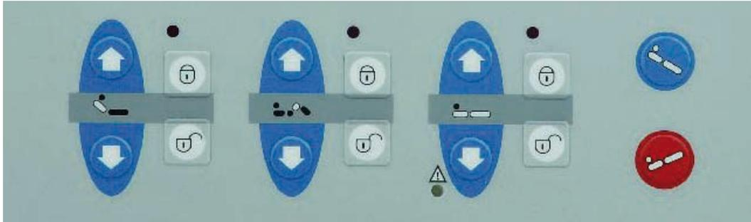
● The LED lights up red if the up or down button is pressed while the drive is locked.
