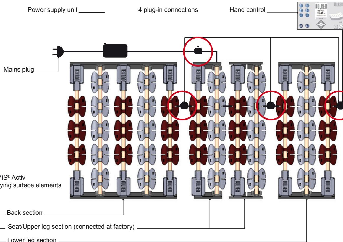
When using the MiS® Activ in a Vis-a-Vis bed, please note that the additional Vis-a-Vis adapter cable has to be inserted between the upper and lower leg section.
