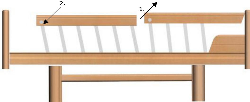
To lower the side rails, press the button at the lower part of the respective element (2) and move the side rail downwards. Start with the part of the side rail on the footside of the bed.
