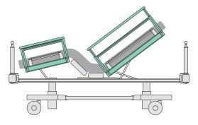
The head and torso are protected at all times due to the moving side rail – even when the upper body section is raised.
