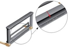
3. Push the rail element completely underneath the lying surface.
