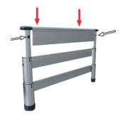
2. To lower the side rail further, raise the side rail slightly using the longitudinal profiles to release the lower catch. At the same time, push the two outer locking knobs in and slide the middle section down into the lowest position.
