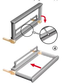
When using the elevated side rails (43.5 - 45 cm), the mattress holders must be opened before raising the rails and closed again after the rails have been retracted (not illustrated).
