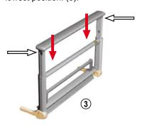
Press the trigger labelled "Drücken/Press" at the bottom of the assist rail. Then tilt the rail until it is horizontal and parallel with the floor. Slide in the side rail until it is fully retracted under the lying surface (4).
